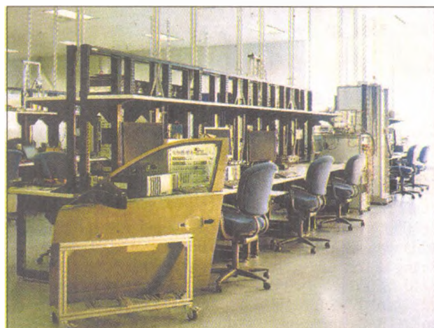
Bosch's lab in Plymouth Township, part of its Farmington Hills-based automotive technology group, puts a variety of the company's car and truck components, such as a window lift that might go into this car door, through extreme conditions. The lab includes a machine shop for internal use, but no auto parts are manufactured on the site.
