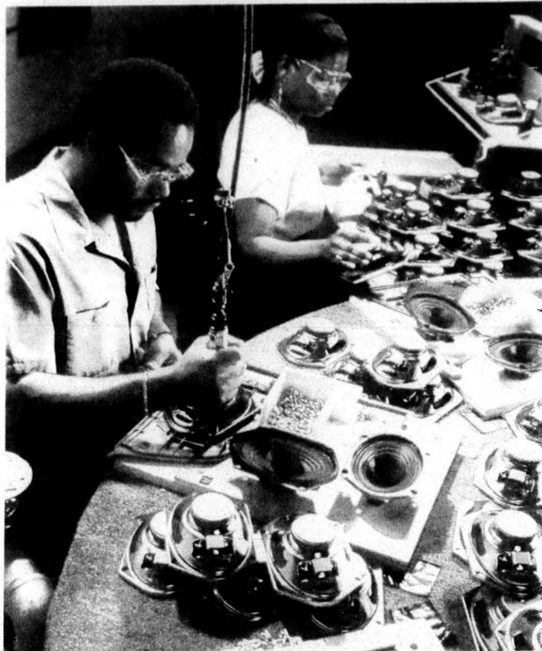
Final assembly: Workers at Jensen's Livonia plant add the last components and give one more test to speakers destined for Ford vehicles.
