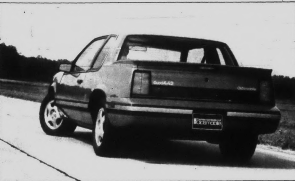
The 1991 limited edition Oldsmobile Cutlass Calais Quad 442 includes an enhanced Quad 4 engine, a special transaxle, fuel system improvements and anti-lock brakes.
