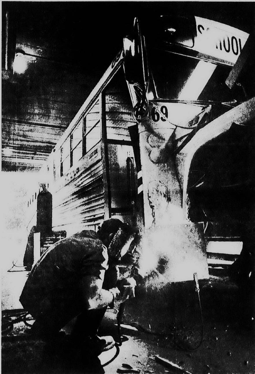
David Pathe patches cracks on a bus. Heavier metal is being welded to withstand stress because the front corner acts as a snowplow during winter.
