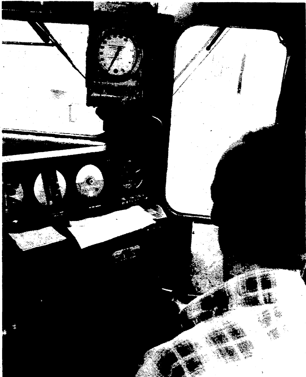
AN ENGINEER'S EYE VIEW from engine no. 4296, on its way from the Eckles Road crossing to Toledo. Various controls at the console regulate and measure current from the diesel-powered generator to axle motors; pressure to brakes; and myriad other engine, generator and drive functions. (Crier photo by Robert Cameron)
