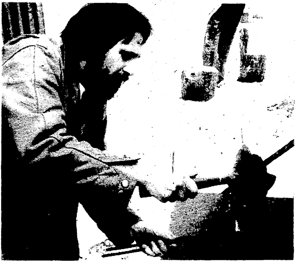
STEP TWO. John Stanford prepares the shoe, heating it in a portable forge in his pick-up truck, and hammering it into shape.
